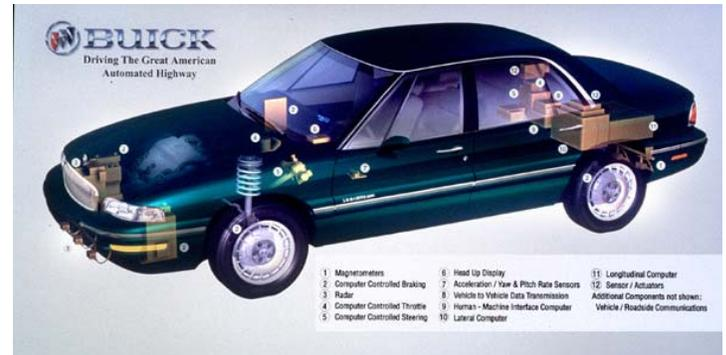
Figure 6. Experimental test vehicles.
